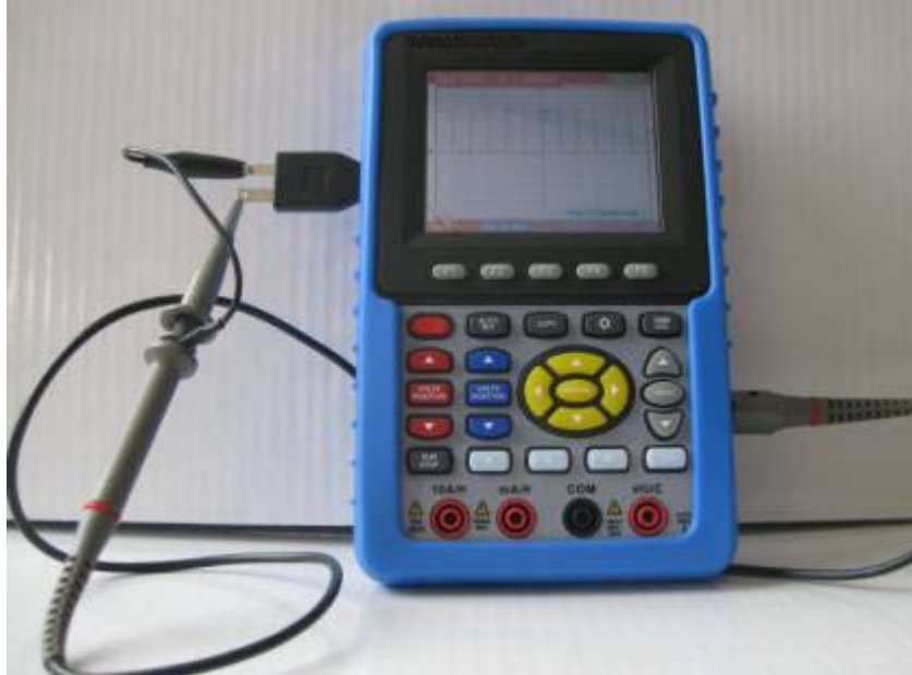
Fig.3. The connection of Square-wave test signal
