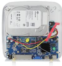
3) Connect data wire and HDD wire between PCB board and HDD.
