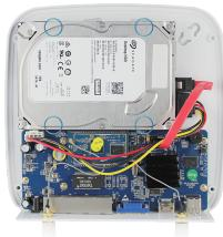
2) Fix the HDD on the bottom panel with screws.
