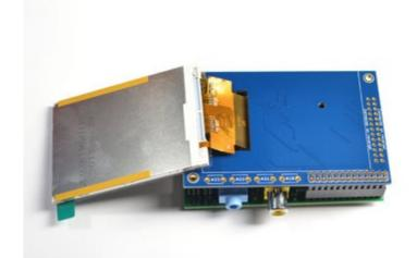
Place the PiTFT shield on top so all the pins stick through the connector on the side. Gently flip the TFT so its off to the side and wont be in your way while you solder
