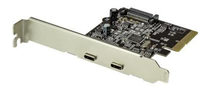
This USB 3.1 card lets you add two USB-C<sup>™</sup> ports to your computer, through a PCI Express slot. It enables you to upgrade your current system by adding two USB 3.1 Gen 2 ports to your computer and giving you access to data transfer speeds up to 10Gbps.
