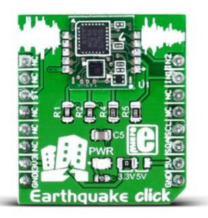
**Earthquake click** carries <u>D7S</u>, the world's smallest high-precision seismic sensor from Omron.
