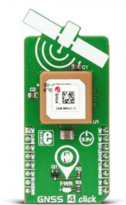
**GNSS 4 click** carries [SAM-M8Q](#) patch antenna module from u-blox.
