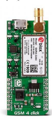
**GSM 4 click** is a mikroBUS<sup>™</sup> add-on board that features the u-blox <u>SARA-G3</u> series 2.5G GSM/GPRS cellular quad-band module.
