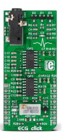
This is an ECG (or EKG) machine on a click board. It measures the electrical activity of a beating heart through electrodes taped to the skin. The board requires little setup, and the final measurement results can be displayed as an Electrocardiogram using a free Windows app.
