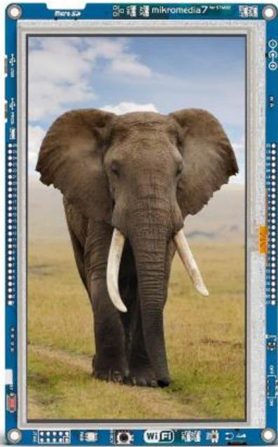
Vivid 7" 800x480px touch screen and over 30 on-board modules, including Ethernet, WiFi and ICD1 debugger all packed onto a single board. Everything is orchestrated by the mighty [STM32F746ZG](#) ARM Cortex-M7 microcontroller family.
