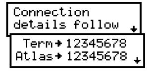
As can be seen from the display here, the connections are verified as being those relating to a normal straight through patch cable. The connections between the *Atlas IT* Terminator end of the cable are shown together with the corresponding he network cable
