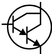
If the device is a Darlington transistor (two BJTs connected together), the unit will display a similar message to this:
