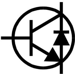
For NPN transistors, the anode of the diode is connected to the emitter of the transistor. For PNP transistors, the anode of the diode is connected to the collector of the transistor.
