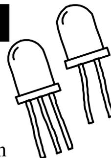
A two terminal bicolour LED consists of two LED chips which are connected in inverse parallel within the LED body. Three terminal bicolour LEDs are made with either common anodes or common cathodes.
