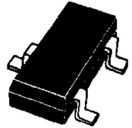
The *Atlas DCA* will intelligently identify popular types of three terminal diode networks. For three terminal devices such as SOT-23 diode networks, the three test clips must all be connected, any way round. The instrument will identify the type of diode network and then display information regarding each detected diode in sequence. The following types of diode networks are automatically recognised by the *Atlas DCA*:
