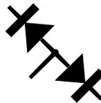
Anodes of each diode are connected together, the BAW56W is an example.
