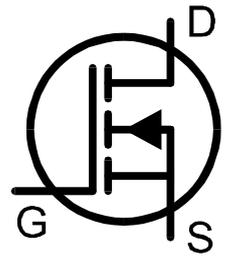
MOSFET stands for *Metal Oxide Semiconductor Field Effect Transistor*. Like bipolar transistors, MOSFETs are available in two main types, N-Channel and P-Channel. Most modern MOSFETs are of the Enhancement Mode type, meaning that
