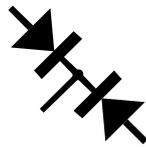
Both cathodes connected together, such as the BAV70 device.
