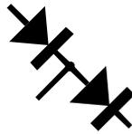
Here, each diode is connected in series. An example is the BAV99.
