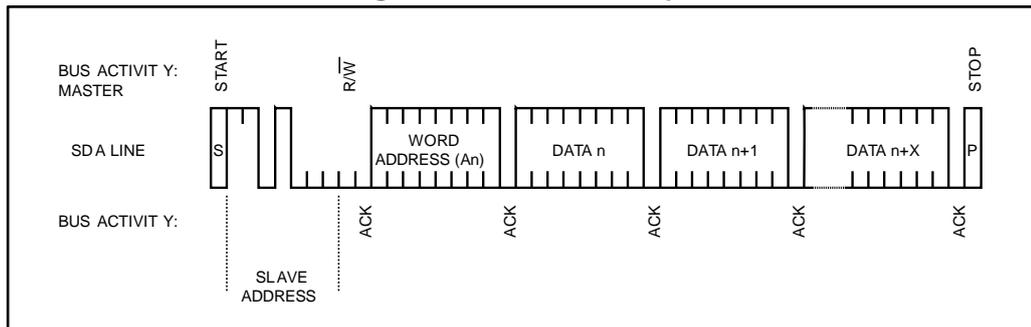
Figure 13: WRITE cycle timing: RTC and external SRAM control signals
