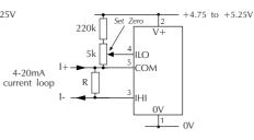
Measuring a 4-20mA loop current.
