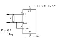
Measuring current. The meter's supply is isolated from the current being measured.
