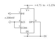
Measuring an input voltage referenced to a floating supply, i.e. the input voltage and the meter's power supply are isolated from each other. Circuit shows DP1 enabled.
