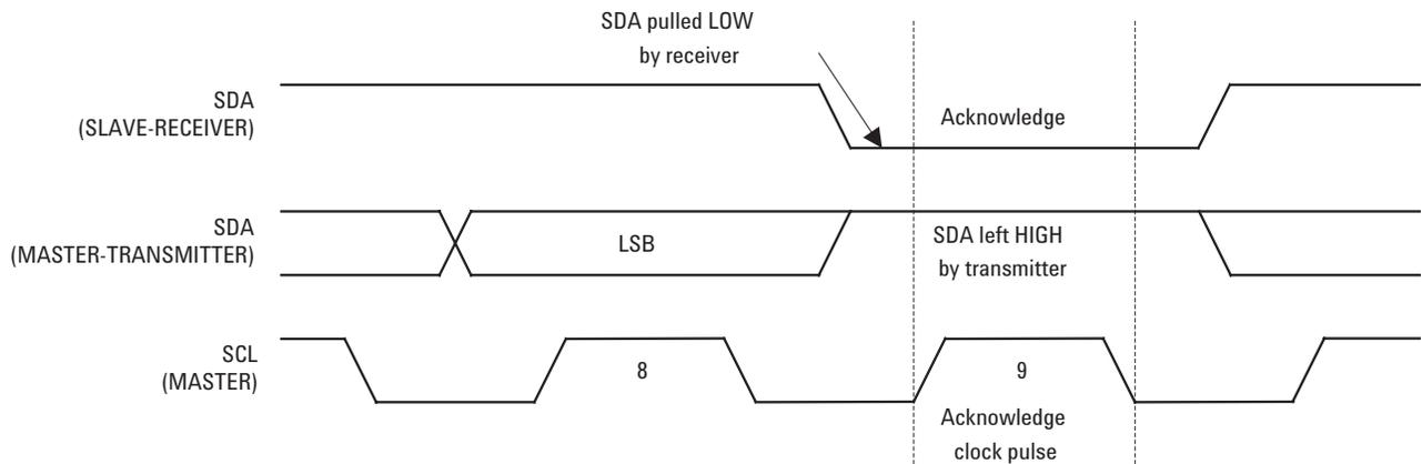
**Figure 6. Slave-Receiver Acknowledge**
