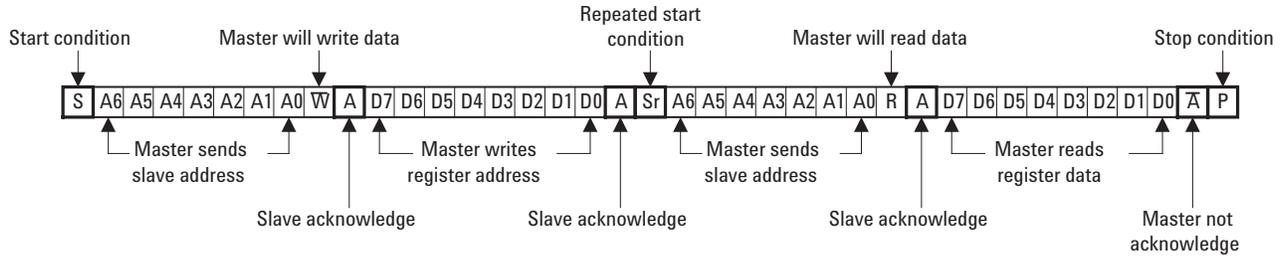
Figure 10. Register Byte Read Protocol
