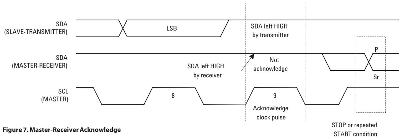
**Figure 7. Master-Receiver Acknowledge**
