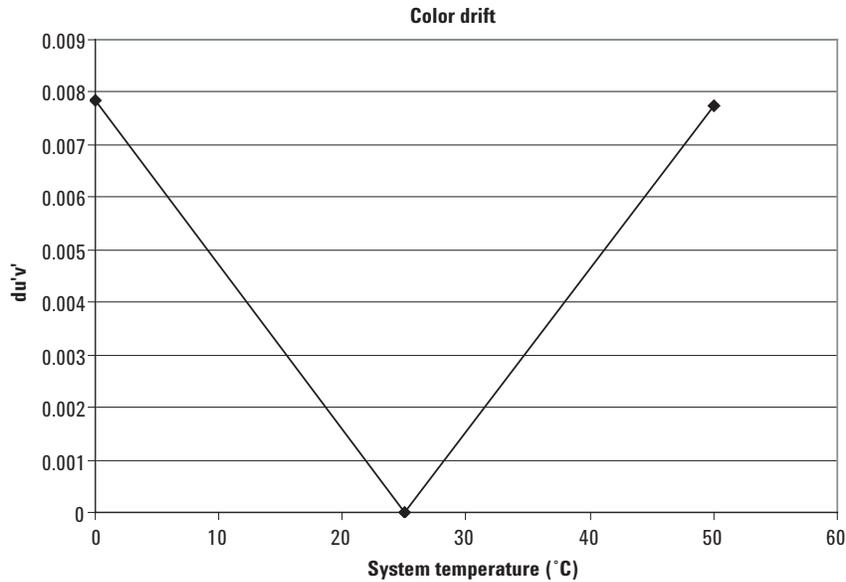
Note: The starting point is at 25°C and is zero color drift as all measurements are made relative to the starting point at 25°C.
