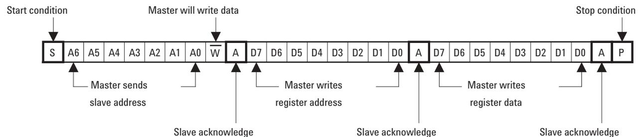
**Figure 9. Register Byte Write Protocol**
