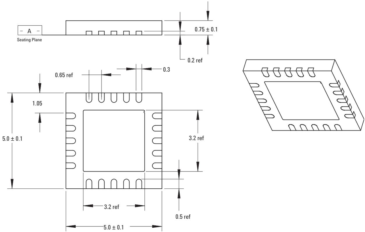
Note: Dimensions are in millimeter (mm)
