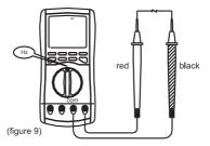
The measurement ranges are: 4.000kHz, 40.00kHz, 40.00kHz, 400.0kHz, 4000MHz, 40.00MHz and 400.0MHz. To measure frequency, connect the Meter as follows:
