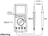
Never attempt an in-circuit current measurement where the open-circuit voltage between the circuit and ground is greater than 250V.
