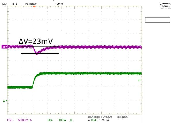
Step Load Transient Response (Vin=5.0V, Vout=1.8V, Load=660uF,
