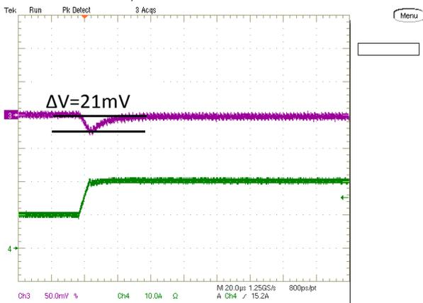
Step Load Transient Response (Vin=5.0V, Vout=0.7V, Load=660uF,
