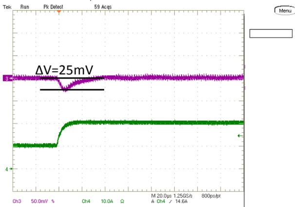
Step Load Transient Response (Vin=12.0V, Vout=1.8V, Clod=660uF,
