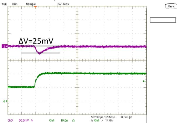
Step Load Transient Response (Vin=12.0V, Vout=1.0V, Cload=660uF, Iout=20A to 10A, 2.5A/us) Trace 3=Vout, 50 mV/div, Trace 4=Iout, 10A/div.
