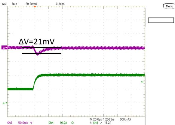
Step Load Transient Response (Vin=5.0V, Vout=1.0V, Load=660uF,
