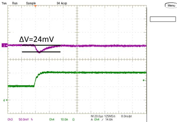
Step Load Transient Response (Vin=12.0V, Vout=0.7V, Cload=660uF,
