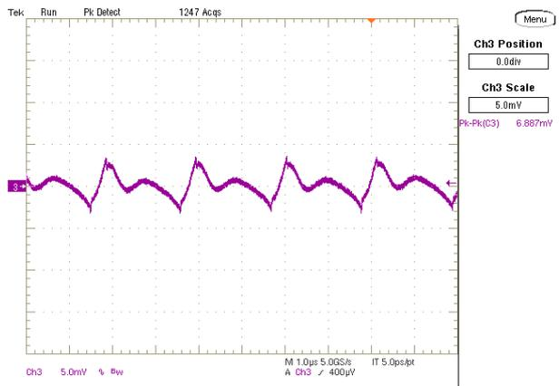
Step Load Transient Response (Vin=5.0V, Vout=0.7V, Load=660uF,
