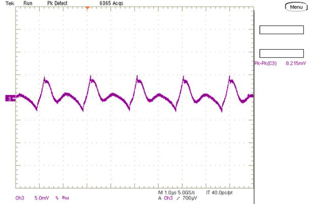
Step Load Transient Response (Vin=12.0V, Vout=1.8V, Clod=660uF,
