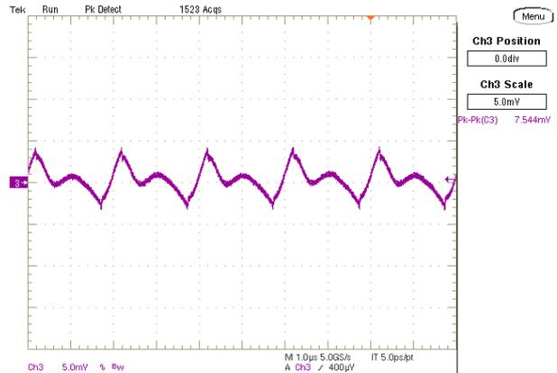
Step Load Transient Response (Vin=5.0V, Vout=1.0V, Load=660uF,
