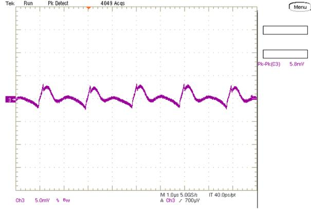
Step Load Transient Response (Vin=12.0V, Vout=1.0V, Cload=660uF, Iout=10A to 20A, 2.5A/us) Trace 3=Vout, 50 mV/div, Trace 4=Iout, 10A/div.
