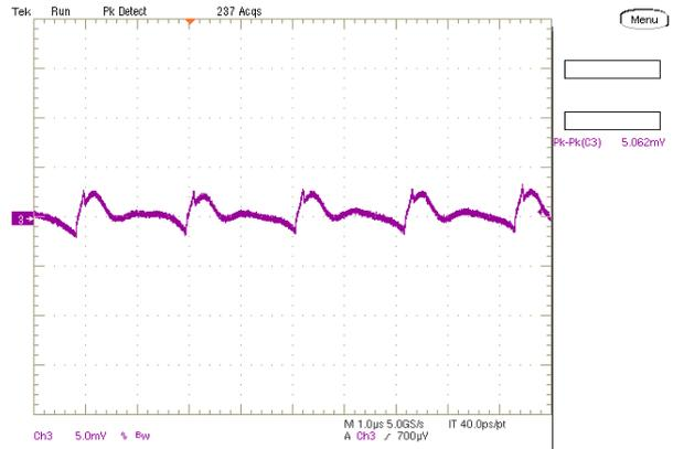
Step Load Transient Response (Vin=12.0V, Vout=0.7V, Cload=660uF,
