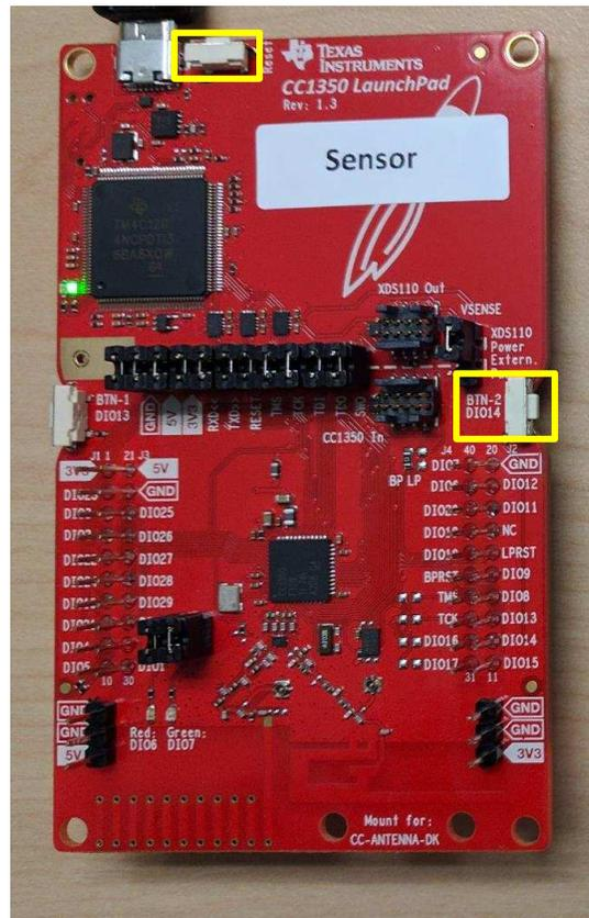
Figure 34. The Reset and BTN-2/DIO014 Buttons are Outlined
