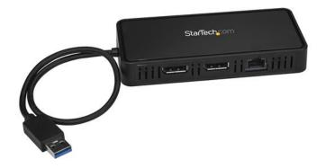
This USB to dual DisplayPort mini docking station makes it easy to create a high-performance dual-4K workstation, connecting your MacBook or Windows® laptop to two DisplayPort monitors plus Gigabit Ethernet wired network. The dock features a compact design that's perfect for business professionals who need a highly functional workstation when working or traveling between multiple office locations, or when using shared workspaces.
