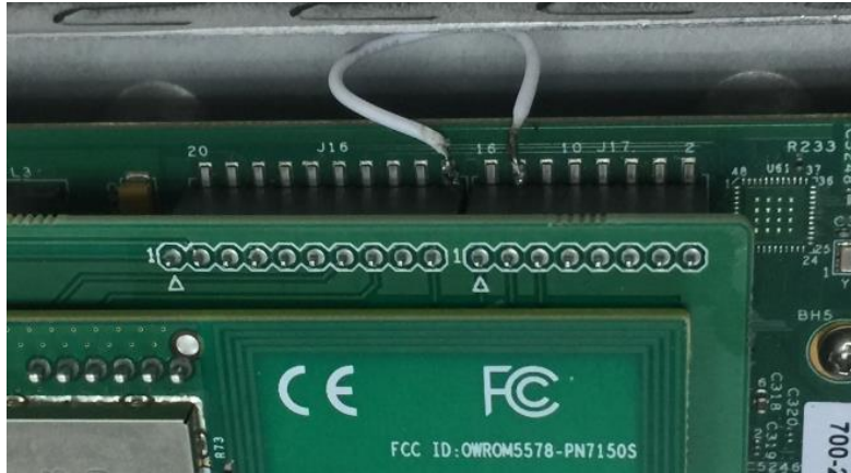
Figure 4-5 NFC hardware rework on LS1012aRDB
