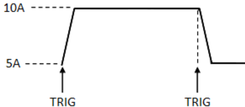
Figure 22 - Toggle Transient Operation
