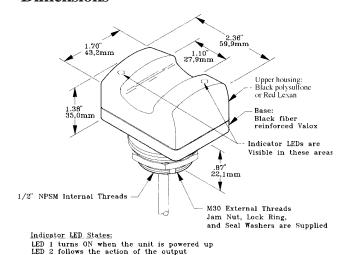
Model shown has built-in, attached cable.
