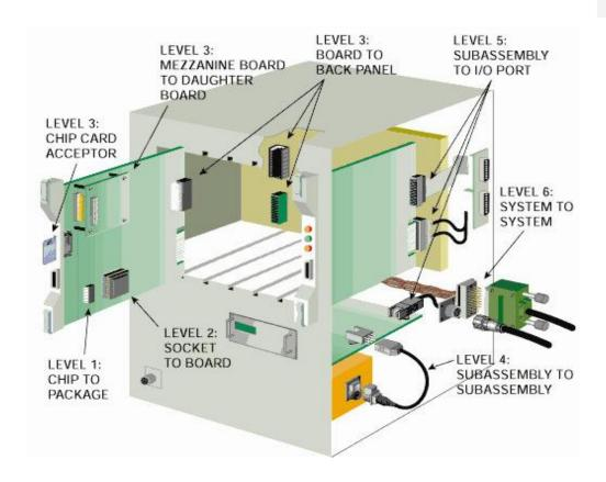
Metral<sup>®</sup> is a system at Packaging Level 3 (Board to Board) with complementary solutions packaging Levels 4, 5 and 6
