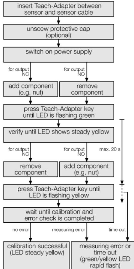
The measuring signal in the sensor is influenced by the diameter and the material characteristics of the center bolt, but also by the cover of the sensitive area. Therefore each sensor has to be conditioned to the operating environment, i.e. to the applied sleeves or protective caps and the target (nut, sleeve etc.) In order to calibrate a sensor, the teach adapter VB2-SP1 made by Turck is needed.
