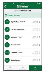
View fault details immediately. All faults are time and date stamped.
