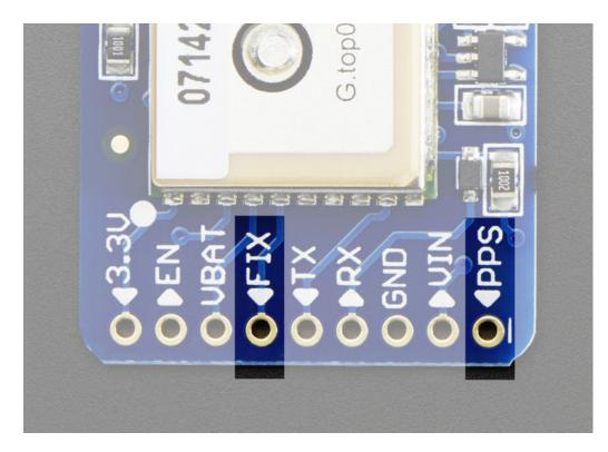
**FIX** is an output pin - it is the same pin as the one that drives the red LED. When there is no fix, the FIX pin is going to pulse up and down once every second. When there is a fix, the pin is low (OV) for most of the time, once every 15 seconds it will pulse high for 200 milliseconds
