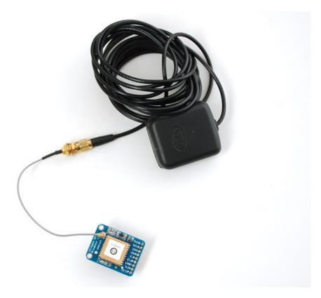
All Ultimate GPS modules have a built in patch antenna - this antenna provides -165 dBm sensitivity and is perfect for many projects. However, if you want to place your project in a box, it might not be possible to have the antenna pointing up, or it might be in a metal shield, or you may need more sensitivity. In these cases, you may want to use an external active antenna.
