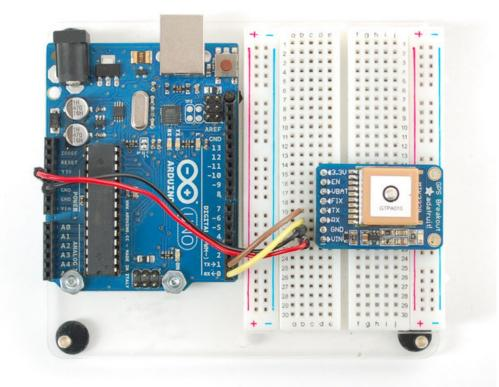
Now plug in the USB cable, and open up the serial monitor from the Arduino IDE and be sure to select **9600 baud** in the drop down. You should see text like the following:
