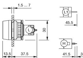
L1 = Solder/Plug-in terminal 2.8 x 0.5 mm
