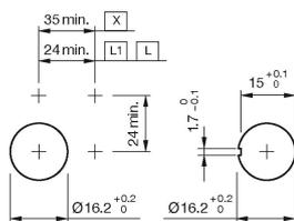
L1 = Solder/Plug-in terminal 2.8 x 0.5 mm
