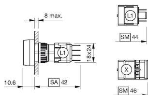
L1 = Solder/Plug-in terminal 2.8 x 0.5 mm
