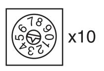
On the upper rotary switch x10, use a small screwdriver to set the tens digit for the address ("3" in the example).
