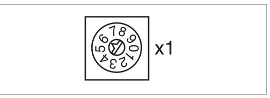
• On the lower rotary switch x1, set the ones digit for the address ("6" in the example). Station address 36 is set in the diagrams as an example.
