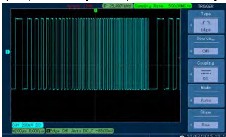
Figure 4- 132 Observe frequency sweep waveform with oscilloscope
