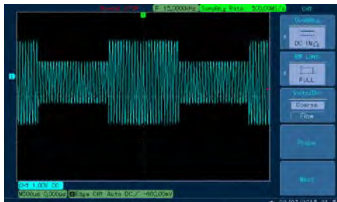
Figure 4- 46 Observe ASK waveform with oscilloscope
