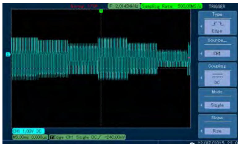
Figure 4- 98 Observe QAM waveform with oscilloscope
