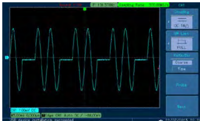
Figure 4- 145 Observe BURST waveform with oscilloscope
