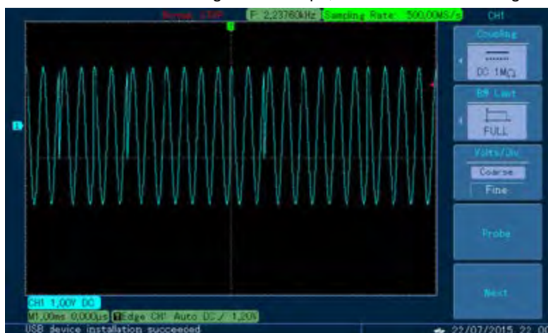
Figure 4- 72 Observe BPSK waveform with oscilloscope
