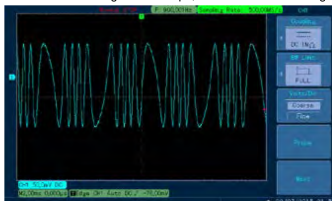
Figure 4- 36 Observe PM waveform with oscilloscope
