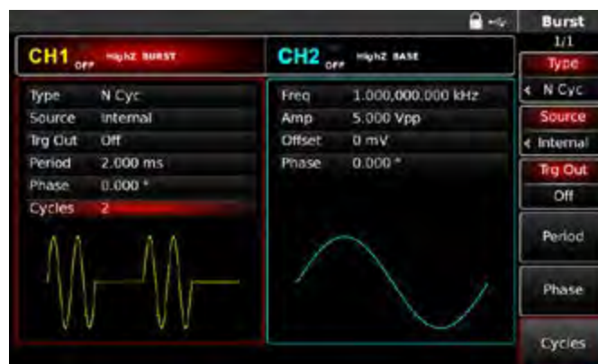
Figure 4- 139 Set N cycle function
