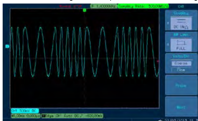
Figure 4- 55 Observe FSK waveform with oscilloscope
