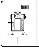
Flashing of digits shows a flat battery.
