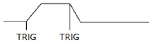
This example assumes that CC mode is active, the slew rate is at the factory default setting (maximum rate) and a trigger signal is connected to the mainframe's external trigger input. Toggle transient operation is similar to that described for continuous and pulse operation, except that each time a trigger is received the input alternates between the level A and level B current levels.
