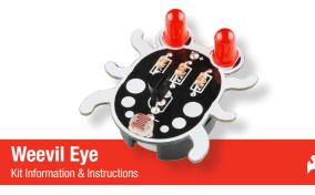
The Weevil Eye kit is an introductory electronics kit designed to help the novice electronics enthusiast learn about things like soldering and resistance. The Weevil Eye is designed to look like a little beetle whose eyes glow in accordance with the ambient light level – the less light detected, the brighter the friendly weevil's eyes will glow. There is no programming involved and all soldering is beginner friendly, so this kit is perfect for the embedded electronics novice.
