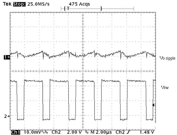
Figure 14. The Output Voltage Ripple Using One 100  $\mu$ F POSCAP Capacitor
