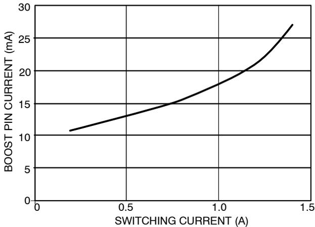
**Figure 7. The Boost Pin Current Includes 7.0 mA Pre-Driver Current and Base Current when the Switch is Turned On. The Beta Decline of the Power Switch Further Increases the Base Current at High Switching Current**
