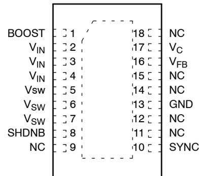
Note: DFN exposed pad may be soldered to a heat spreader for enhanced thermal performance. The exposed pad may be connected to GND; do not connect to any other potential.
