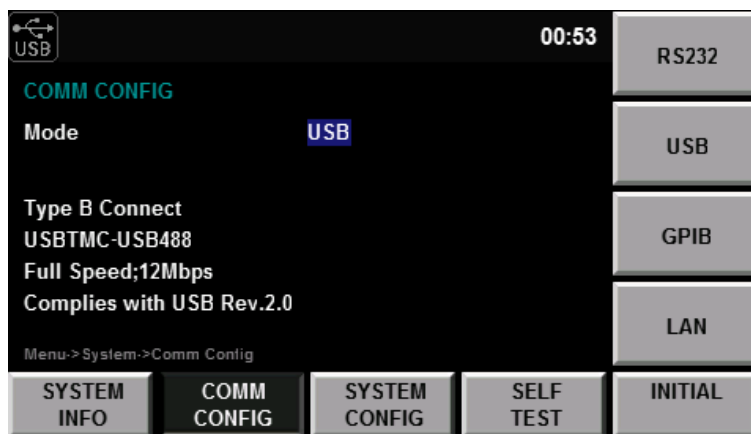
Figure 2.4: COMM Configuration - USB
