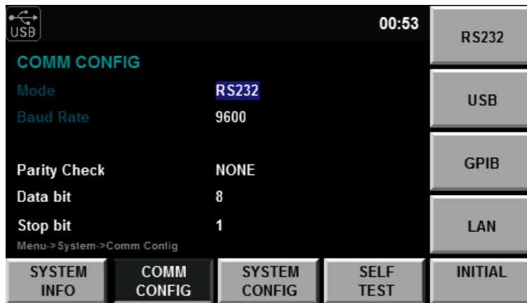
Figure 2.3: COMM Configuration - RS-232
