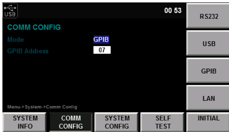
Figure 2.5: COMM Configuration - GPIB
