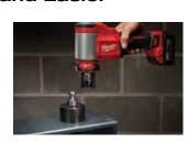
Step 1: Set up Bold crosshairs and a clear view of the work surface make alignment fast and easy
