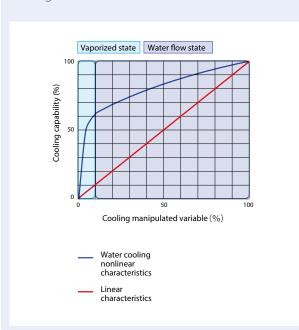
It constantly detects changes in the temperature behavior and suppresses the temperature variation by automatically adjusting the proportional band (cooling).
