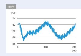
When sensor is placed closer to sealing surface, sometimes periodic temperature variation is caused by the heat switching on and off during the sealing period.
