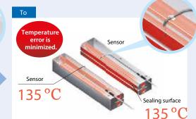
Sensor is able to acquire real temperature sensor surface.
