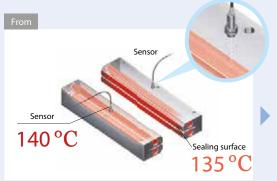
Cause not perfect sensor location there is 5°C difference vs temperature sealing surface.
