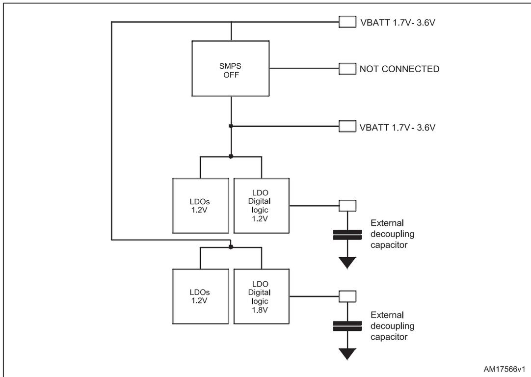
Figure 11: Power management strategy using step-down DC-DC converter
