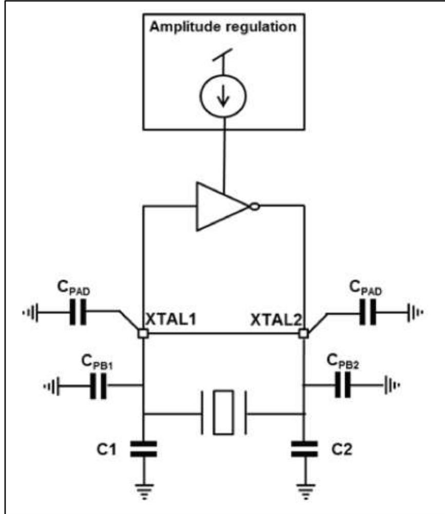
Low power consumption and fast startup time is achieved by choosing a quartz crystal with a low load capacitance  $C_0$ . To achieve good frequency stability, the following equation needs to be satisfied:
