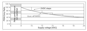
Figure 4: PWM duty ratio as a function of supply voltage with 2VDC step regulation
