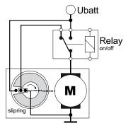
Fig. 3 Wiper with slipring
