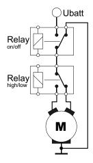
Fig. 4 Dual speed wiper-circuit
