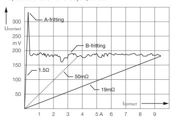
Fig. 2 Fritting of a relay contact
