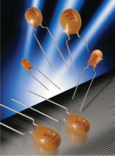
TAP is a professional grade device manufactured with a flame retardant coating and featuring low leakage current and impedance, very small physical sizes and exceptional temperature stability. It is designed and conditioned to operate to +125°C (see page 277 for voltage derating above 85°C) and is available loose or taped and reeled for auto insertion. The 15 case sizes with wide capacitance and working voltage ranges means the TAP can accommodate almost any application.
