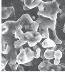
Figure 2. Sintered Anode
