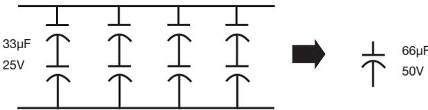
In order to ensure reliable operation, the capacitors should be connected as shown below to allow current sharing of the ac noise and ripple signals. This prevents any one capacitor heating more than its neighbors and thus being the weak link in the chain.
