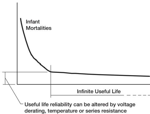
The useful life reliability of the Tantalum and OxiCap® capacitors in steady-state is affected by three factors. The equation from which the failure rate can be calculated is:
