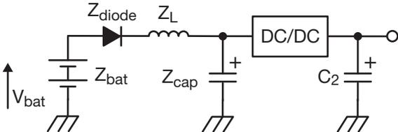
The risk of a high surge current being seen by the capacitor in location C<sub>2</sub> is very small. Therefore if we assume the voltage rail is 2.8 volts and the maximum current seen by C<sub>2</sub> is <1.5 Amps, a 4 volt capacitor could be able to be used in this application.
