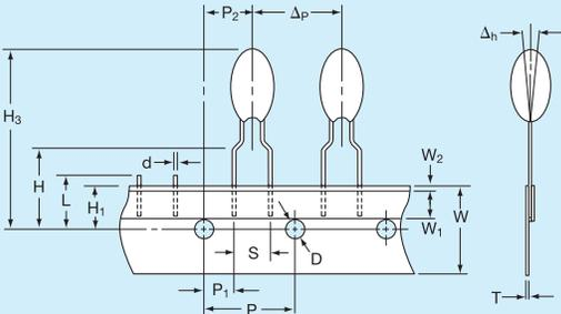
'B' wires for normal automatic insertion on 5mm pitch.
