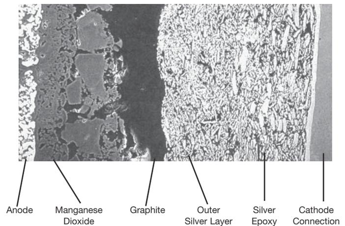
Figure 5. Cathode Termination
