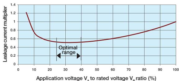
We can identify the range of  $V_A/V_R$  (derating) values with minimum actual DCL as the “optimal” range. Therefore the minimum DCL is obtained when capacitor is used at 25 to 40 % of rated voltage - when the rated voltage of the capacitor is 2.5 to 4 times higher than actual application voltage.
