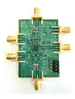
The F1192BEVBI is a fully populated evaluation board which allows the customer to easily evaluate the F1192B. There is on-board 4:1 Balun to translate  $200\Omega$  IF output impedance to  $50\Omega$  for easy evaluation. Jumpers are available for gain control.
