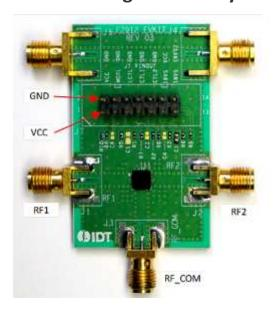
The **F2912EVBI** is the Evaluation Board for High Reliability SP2T RF Switch F2912.
