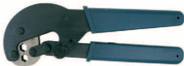
MODEL HX 596Q RG-59, RG-6, and RG-6 Quad Connectors (Hex .324 & .360)
