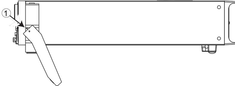
2. After you align the arrows, pull the ends of the handle (1) away from the case.
