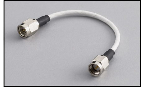
CA-451A: 10.8cm (4.25 in) RG188 coax cable terminated with an SMA male plug on each end, 50 \Omega impedance.
