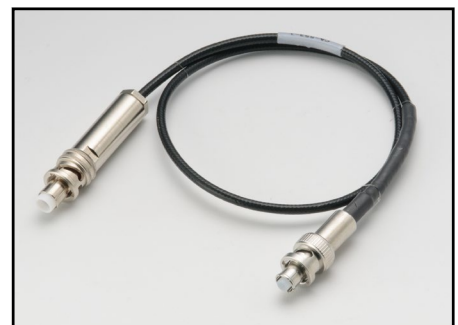
SHV-CA-553-x: High voltage triax to SHV cable (x = 1, 2, or 3m) (3kV rated).
