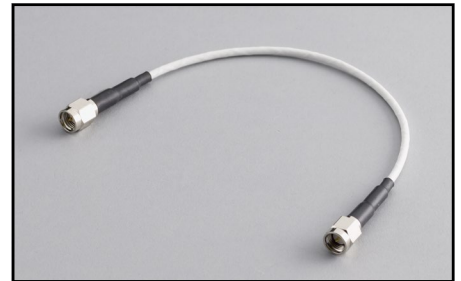
CA-452A: 20.4cm (8 in) RG188 coax cable terminated with an SMA male plug on each end, 50 \Omega impedance.
