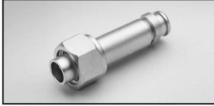
**Model 2188 Low-Thermal Calibration Shorting Plug:** A low-resistance, low-thermal shorting plug required to calibrate the Model 2182A Nanovoltmeter. Made of a LEMO connector with its pin connectors shorted together using copper wire and Sn/Ag4 silver solder.
