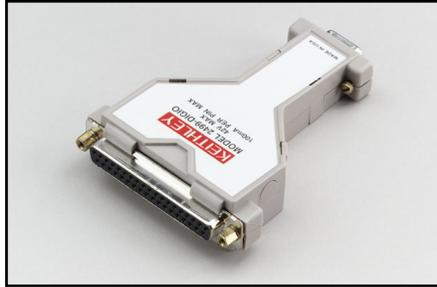
**Model 2499-DIGIO:** Digital I/O expansion module that plugs onto the DB-9 connector of a SourceMeter® SMU instrument. Expands the three digital I/O lines of the SourceMeter to 16 lines. The SOT, EOT/BUSY, 5V, GND, and Interlock signals are passed through.
