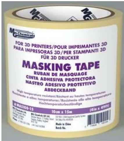
MG Chemicals high temperature masking tape is made of 8 mils thick beige crepe paper coated with a rubber adhesive designed for 3D printer heated beds. It is specifically designed to be heat resistant and provide superior print adhesion while allowing easy removal of completed objects. It also provides protection for the bed, while making clean up simple. It works excellent with PLA, Wood, PETG, and many other 3D printing materials. It is available in 4 in. and 8 in. on 49 ft rolls
