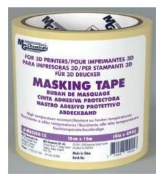
MG Chemicals high temperature masking tape is made of 8 mils thick beige crepe paper coated with a rubber adhesive designed for 3D printer heated beds. It is specifically designed to be heat resistant and provide superior print adhesion while allowing easy removal of completed objects. It also provides protection for the bed, while making clean up simple. It works excellent with PLA, Wood, PETG, and many other 3D printing materials. It is available in 4 in. and 8 in. on 49 ft rolls
