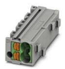
Marshalling patchboard, nom. voltage: 500 V, nominal current: 17.5 A, cross section: 0.14 mm² - 2.5 mm², AWG: 14 - 26, connection method: Push-in connection, number of positions: 1, number of connections: 4, width: 11 mm, length: 8.6 mm, color: gray, color of connection elements: green, mounting: for snapping onto a DIN rail adapter, for snapping onto a cover flange
