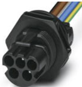
PRC device connector, black, 5-pos., 690 V (IEC 61984), 32 A, crimp connection, 4.0 mm 2 with 150 mm cable length, cut smooth at the end
