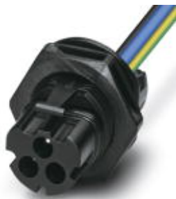
PRC device connector, black, 3-pos., 690 V (IEC 61984), 24 A, crimp connection, 2.5 mm 2 with 150 mm cable length, cut smooth at the end
